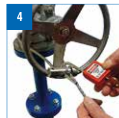
Place padlock through the centre hole
