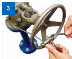
Tighten the tamper proof screw with the special tool provided
